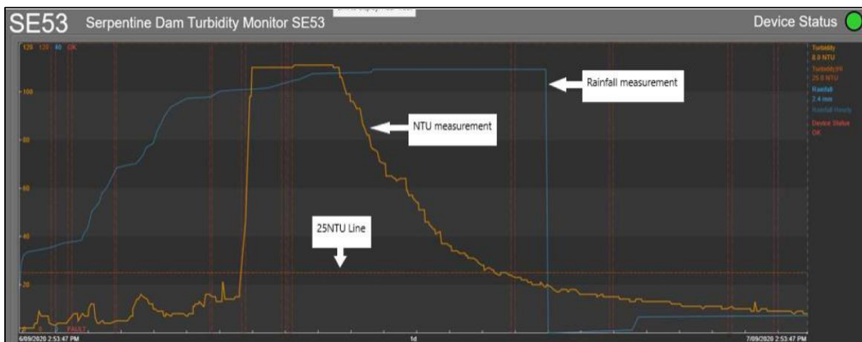
Figure 2: Typical ‘true’ exceedance event showing the sharp incline and gradually return to background levels.
