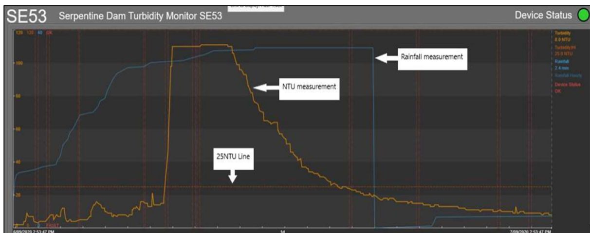
Figure 1 Typical 'true' exceedance event showing the sharp incline and gradual return to background levels.
