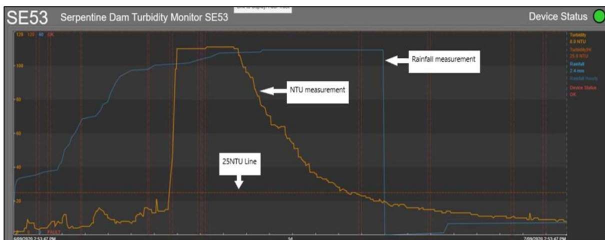
Figure 1 Typical 'true' exceedance event showing the sharp incline and gradual return to background levels.
