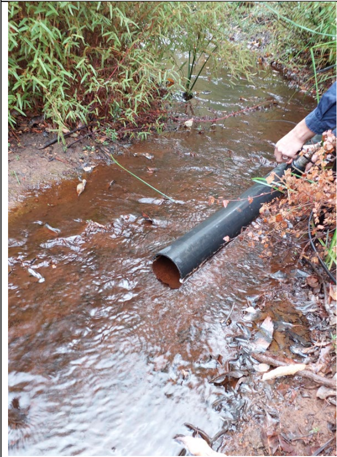
SE02 turbidity monitor in stream with pipe
