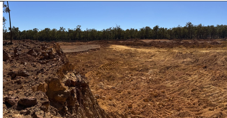
Sections of the Martin 3 are under mining and the pit acts as sump and no immediate drainage risk.
