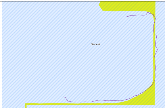
Stone 6 pit boundary walk track (The relinquished FCA width along the eastern and southern edges was 2 m. GPS accuracy was 3 m)
