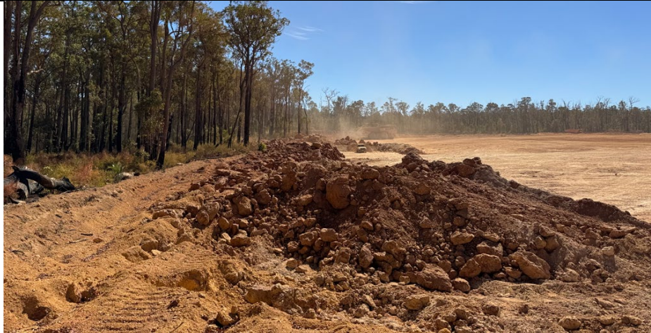
Active mining in Wills 2. The mine face acts as drainage control currently.
