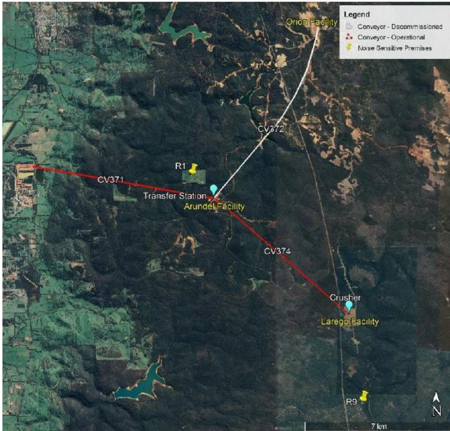
Figure 5: Willowdale mine ore conveyor infrastructure and nearest noise sensitive premises (R1)
