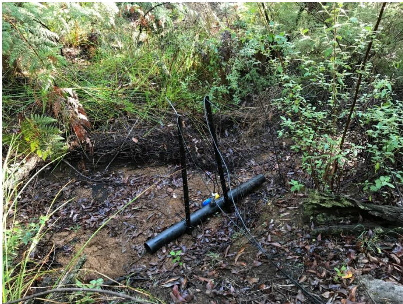
Figure 1. Turbidity monitor located within stream channel.
